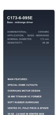
The C173 - 6 - 095E is a 6.5 inch bass-midrange driver with ultra hard ceramic dome.
